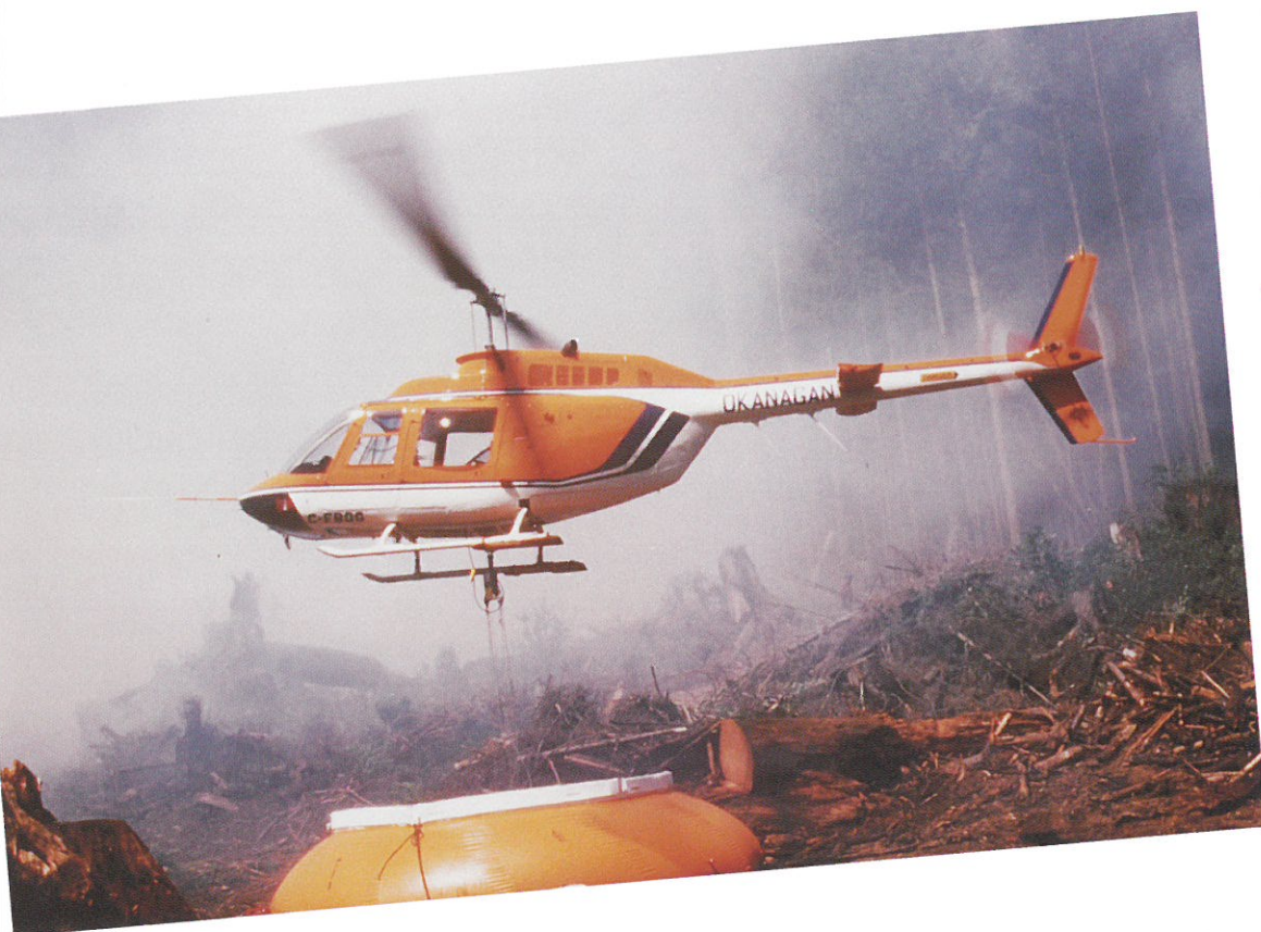
▲ Fixed wing airplanes and helicopters have become cost effective weapons in combatting wildland-type fires when they use foam. Dropping water which contains Phos-Chek foam concentrate onto these fires has been reported to double the effectiveness of these firefighting aircraft.
