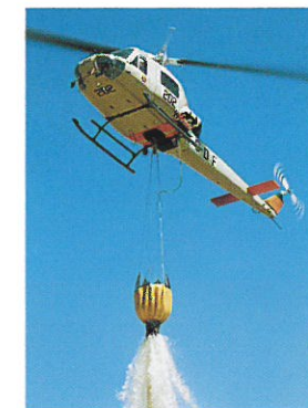
▼ Foam can double the effectiveness of helicopters. More water can be applied faster than with hand-lines, especially in remote, rugged terrain. Longer and more effective fire lines can be built using foam instead of plain water. Foam's visibility allows pilots to see where water has been applied and gauge its coverage.
