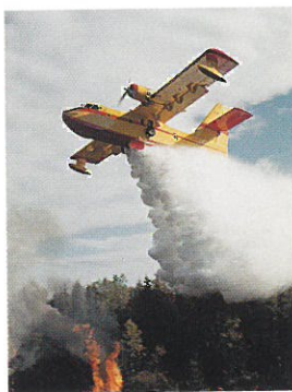
▲ Fixed wing airplanes and helicopters have become cost effective weapons in combatting wildland-type fires when they use foam. Dropping water which contains Phos-Chek foam concentrate onto these fires has been reported to double the effectiveness of these firefighting aircraft.
